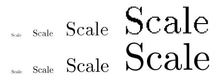
Figure 8.25: Scaling a bitmapped picture (top) and a vector picture (bottom)
