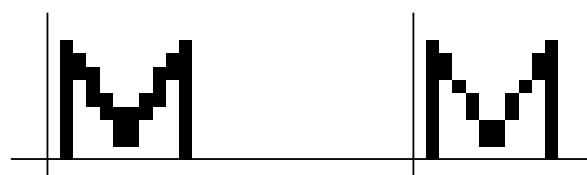
Figure 5 The character on the right has been created with all the define_xxx_pixels commands removed from the source.
