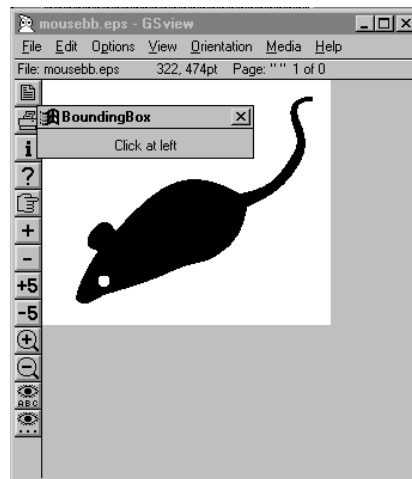
Figure 3 GSview PS to EPS: telling GSview about the boundingbox
