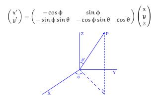
The (full) transformation matrix can be understood as to be composed of 2 rotations: first around the z-axis and second around the transformed x-axis, such that the z-axis coincides with the view direction  $OP \perp$  the new xy-plane. We can omit the  $3^{rd}$ , the transformed z-coordinate, because it is no longer visible in the (orthogonal) projection. The factorization of the projection matrix is
