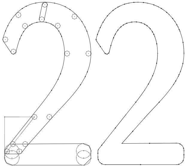
Figure 3. The glyph of the numeral 2 in xmssdc10 font. We can see envelopes and pens (thick curves) and a contour (thin curve).
